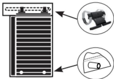
Before installing the motor, be sure that the upper safety blocks and lower stoppers are present on the window.
